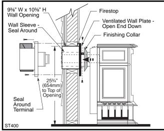
Fig. 19 PDV20 with Rear Vent Kit 7TFSRSK installation.
